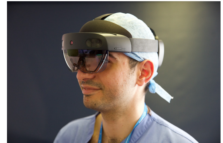
Figure 2. The HoloLens 2 Headset. It consists of a mounted computer (at rear of the head), a visor which projects holographic images on the user’s eye. It also contains a forward-looking camera in the centre of the headset and sensors mounted at the front on each side. Finally, it possesses a noise cancelling microphone for voice communication.
